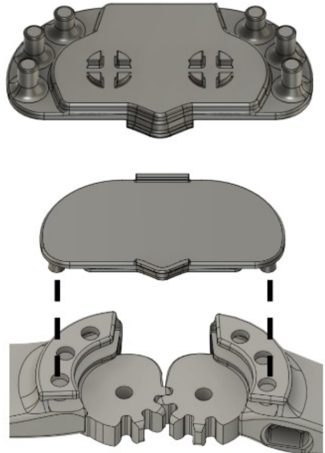
Figure 1. At the top we see the underside of the hinge cap that is then flipped over and guided into the gear housing which allows for complete inhibition of
