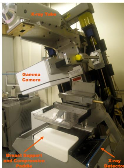
Figure 5-1: Dual Modality Tomosynthesis system (DMT). X-ray tube, gamma camera, and x-ray detector are on a single gantry arm which rotates around an independent breast compression system. This allows for x-ray and gamma image registration. The gamma camera shown in this photo is the older, thicker one.
