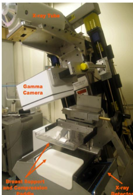
Figure 3-1: Dual Modality Tomosynthesis (DMT) scanner. X-ray tube, gamma camera, and x-ray detector are on a single gantry arm, which rotates around an independent breast immobilization system. In this photo the gamma camera has been pulled away from the gantry arm so that its posterior edge aligns with that of the breast support. This posterior position is used for MBT scanning, but with the camera lowered to be as close as possible to the compression paddle.
