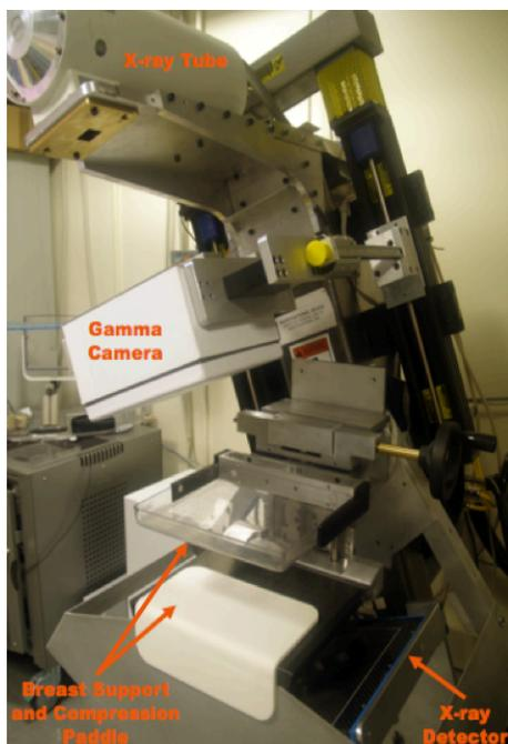
Figure 1-9: Dual Modality Tomosynthesis (DMT) system. X-ray tube, gamma camera, and x-ray detector are on a single gantry arm, which rotates around an independent breast compression system.
