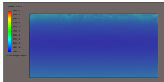
**Figure 25:** A) FEA Setup for Analysis, with Stress Plot B) Visual Stress distribution along Analyzed Beam Cross Section
