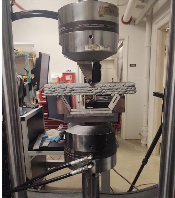
**Figure 18:** 3 Point Bending Flexural Testing Setup
