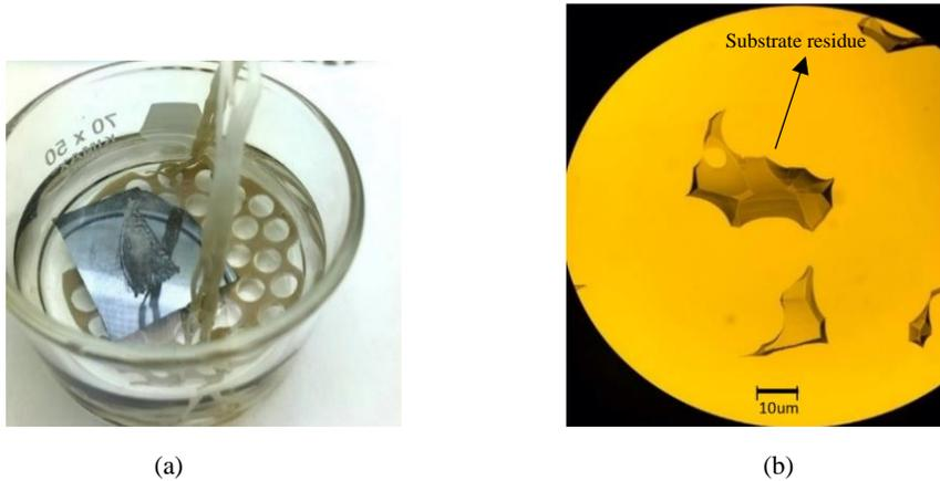
Figure 4-3. (a) Substrate removal of the InP epi bonded onto SOI in hydrochloric acid (b) Substrate residue due to saturated HCL dilution.
