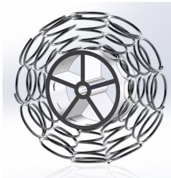
Figure 1: Photograph of Computerized Model of Compliant Foot/Wheel Mechanism
