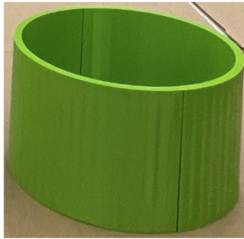
Figure 55. Extended nosecone mold (Height 10 cm)
