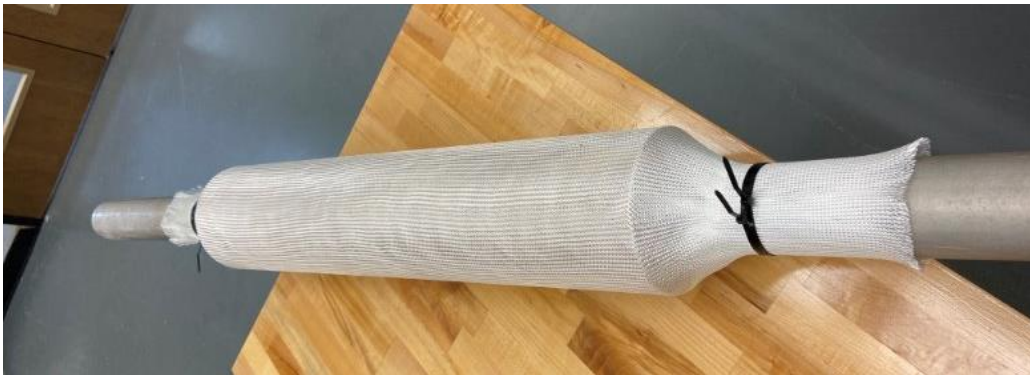
Figure 63. Fiberglass sleeve fixed over phenolic tubing.
