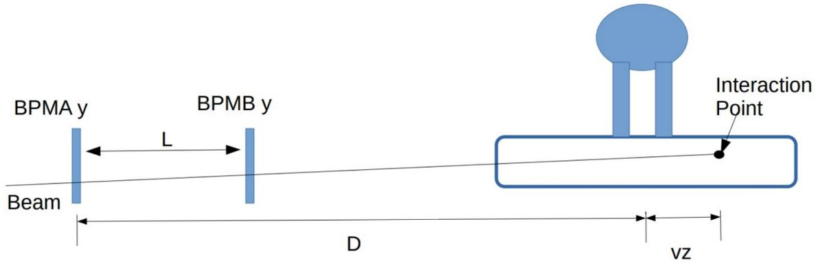
FIGURE 3.12: Diagram of the beam going through the BPMs and reaching the target.
