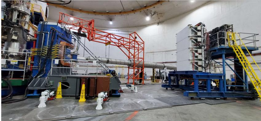
FIGURE 3.9: Picture of the hadron arm in hall A. On the left is the SBS magnet and the right is HCal, located 17 m away.
