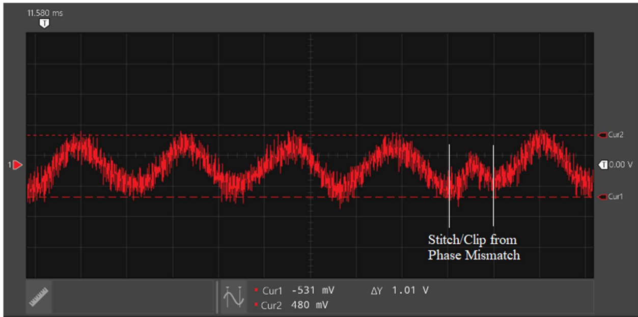
Figure 25: Phase Clipping Between Two Audio Sections
