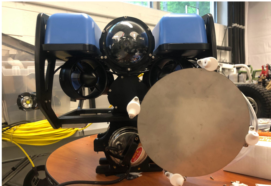
Figure 9: ROV Cleaning System.
