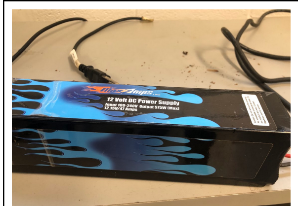
12V DC power supply
