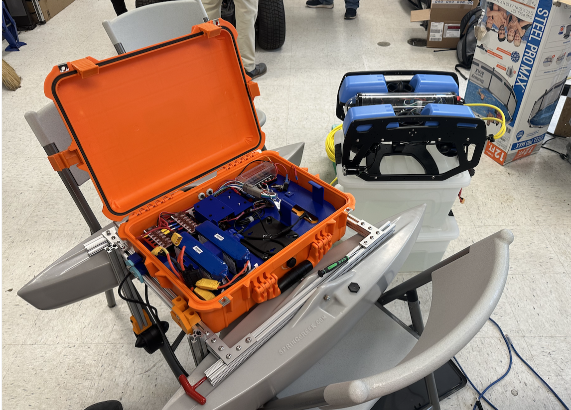
Figure 6: Full overview of the ASV and BlueROV2 system.
