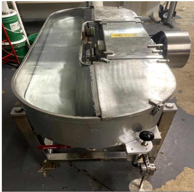
Figure 8: Shows the Hollander beater. The right side houses the maceration mechanism operated by a belt driven turbine. Bottom right of the picture shows the lever that controls the gauge length. The left half of the Hollander beater is open face allowing for pulp consistency to be monitored while pulping is in progress.
