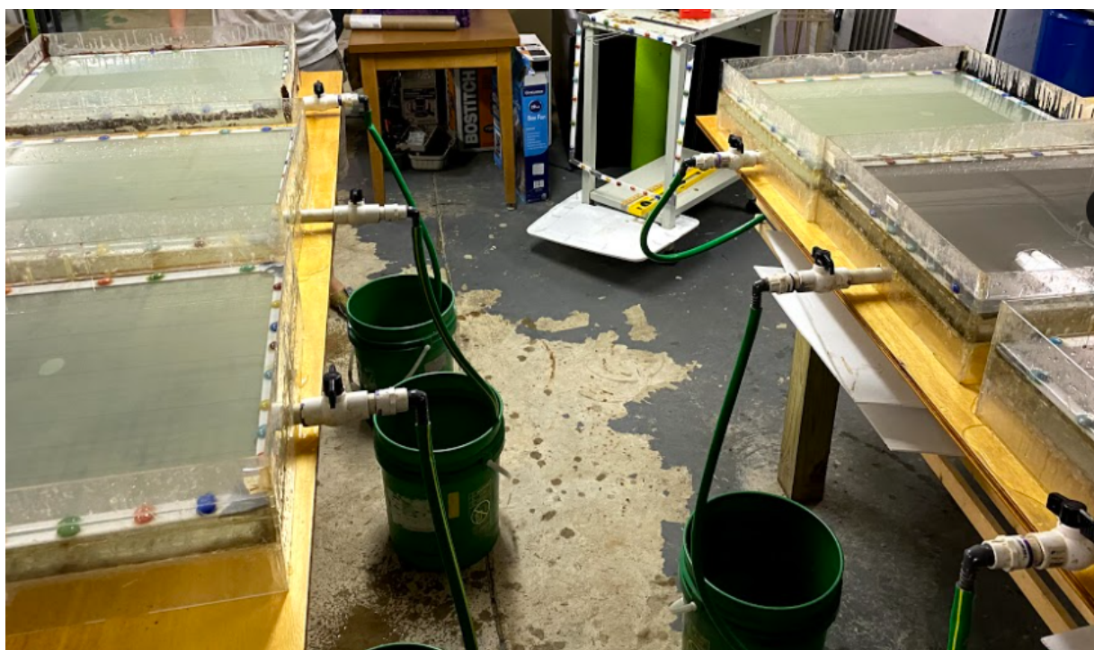
Figure 10: 6 SFCs and recyclable drainage systems set up in parallel pre and post staging with water and border-weighted fourdrinier catching/drying stage.
