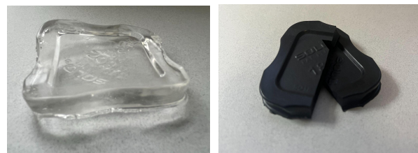
Figure 3: First models of Sylgard 184 and Sylgard 170, left to right. The bottom of a plastic cup was used as a mold.
