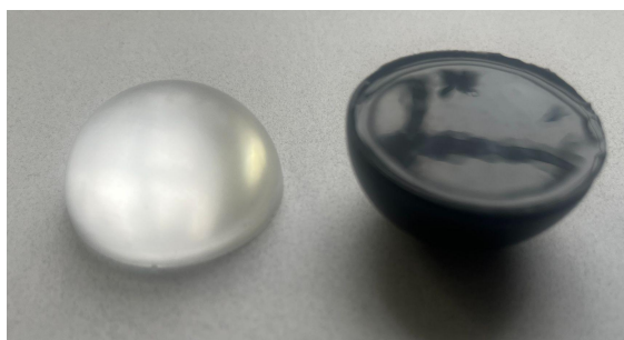
Figure 5: Third models of Sylgard 184 and Sylgard 170, left to right. A table tennis ball cut in half was used as a mold.
