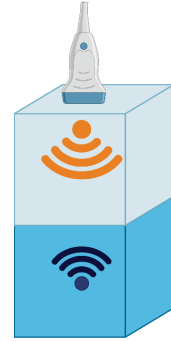
Figure 1: Principle of ultrasound interface. The ultrasonic transducer (top) sends sound waves through the interface material (middle) and into the soft tissue (bottom), where they are reflected back to the transducer and interpreted. If the waves are reflected at the boundary between the interface and the soft tissue, the soft tissue is not able to be imaged.
