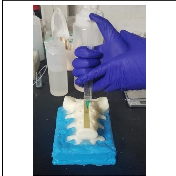
Figure 4: This figure displays the spinal backfilling process. Backfilling of the spinal column is performed to make the phantom realistic and provide consistent results when scanned with the Accuro. Backfilling consisted of inverting the 3-D printed spine onto a silicone mold cast of the top of the spine. The spine was then adhered to the silicone mold using a masking silicone adhesive. Then, a specialized mixture of polyurethane without scatterers was injected through the holes on the bottom of the spine, as shown in this figure.
