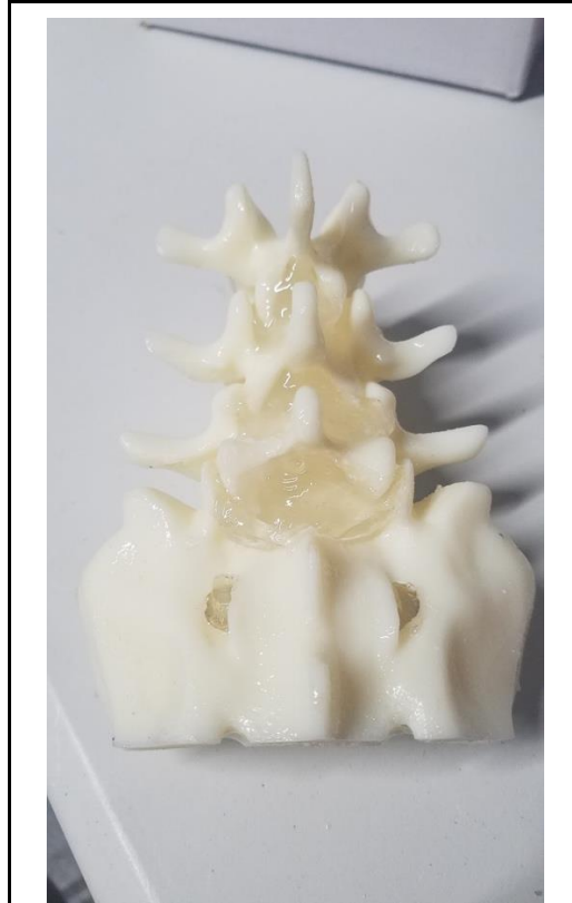
Supplemental Figure 6: The image depicts the backfilled spinal canal. The spinal canal was backfilled with polyurethane. This was done to make the phantom spine more similar to the in vivo human spine.
