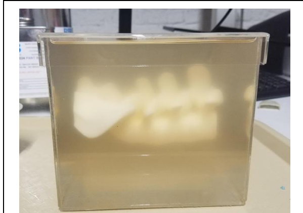
Figure 6: This figure shows a full-scale phantom in a prototype box. The full-scale phantom contains the spine, a stand, the tissue layer, and the skin layer in a prototype box with a lid. Both layers of the phantom are translucent. The 3D printed spine is held in place by a 3D printed, translucent stand, which is difficult to observe from this angle. The prototype box is a plexiglass cube with one open side and a lid. This box will not be used in manufacture of the product because it is not airtight and leaks during the curing process.
