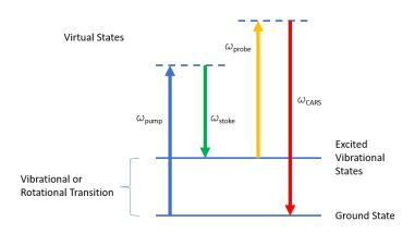
Interaction of Pump, Stokes, and Probe Beam to Produce CARS Signal
