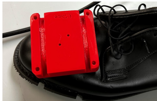
(e) Sensor and marker mount for the thigh for the shoe.
