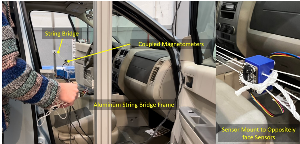
Figure 5.3: The translation of coupled, oppositely-facing magnetometers along string bridge previously used to make insights about magnetic field nonuniformity.
