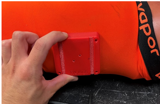
(c) Sensor and marker mount for the thigh.
