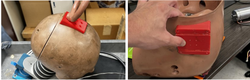
(a) Head mount with placement of magnetometer top rear.
