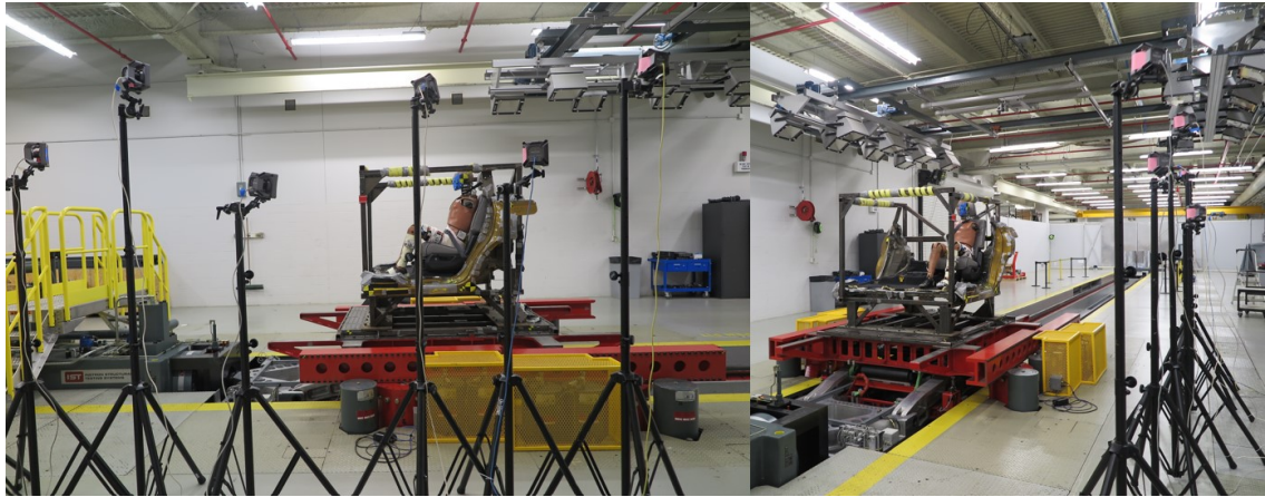
Figure 7.19: The sled buck used for better observing the motion of the test dummy with visual systems during a crash test.
