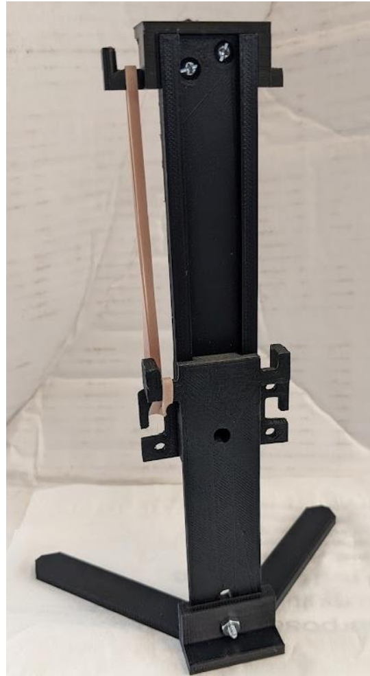
Figure 12: Physical Assembly of Landing Gear
