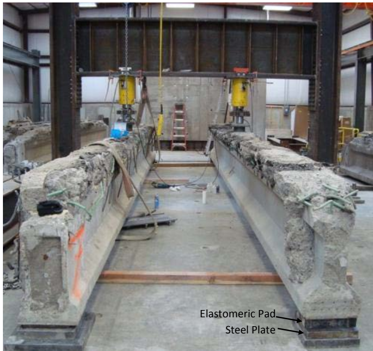
Figure 8 - Phase I Test Setup (Higgs, 2013)
