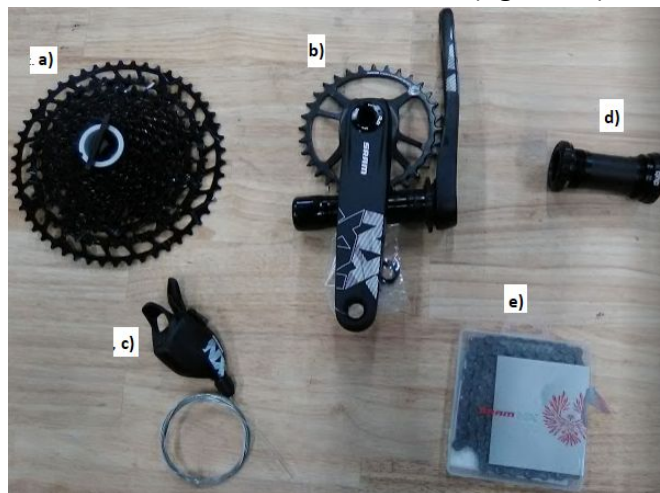
Figure 10: Components in the Groupset. a) cassette, b) crankset, c) shifter, d) bottom bracket, e) chain.
