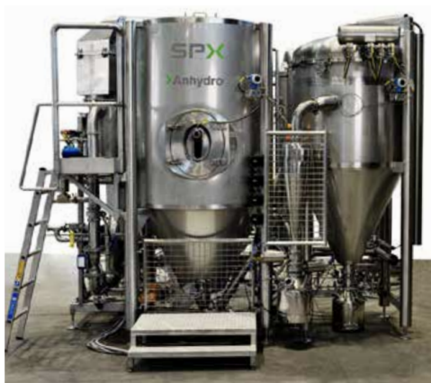
Figure 7.4.2. Pilot Scale SPX Anhydro Spray Dryer
