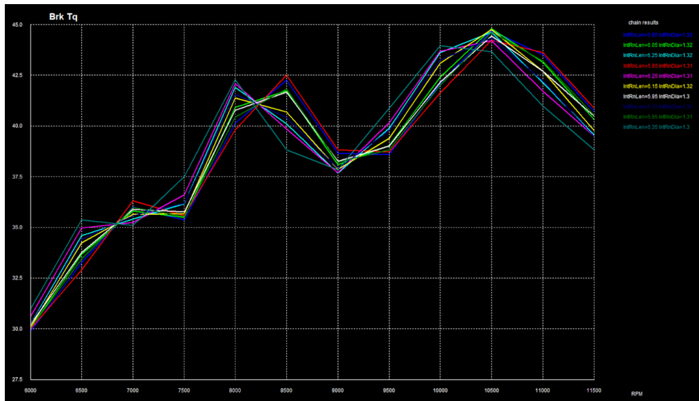
Figure 21. Refined Runner Length and Runner diameter simulation
