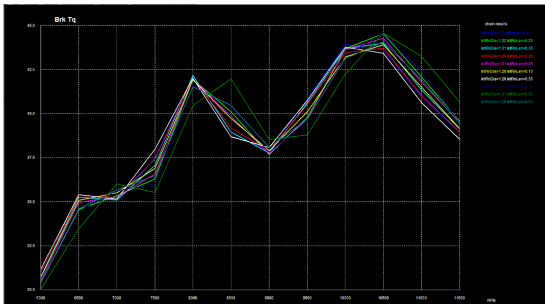
Figure 20. Preliminary Simulation, Runner Diameter and Length variation
