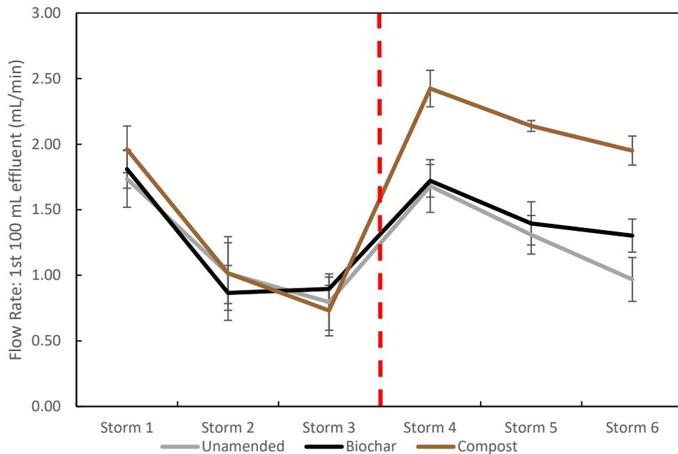
Figure 3-3: Average effluent flow rates, for all columns over entire six-storm series, by treatment type. Error bars represent standard error (n=8 except in for unamended soils in Storms 2, and 3, when one column did not produce 100 mL of effluent; for those data points, n=7). Columns repacked between Storm 3 and 4.
