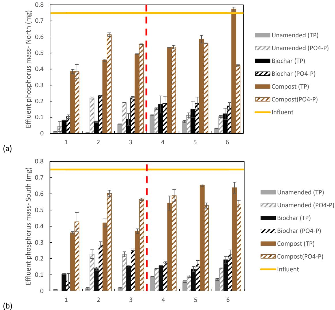
Figure 3-7: Average mass of total phosphorus and phosphate over 6 storm events for north (a) and south (b) regional soils types. Error bars represent standard error (n=2). Columns repacked between Storm 3 and 4.
