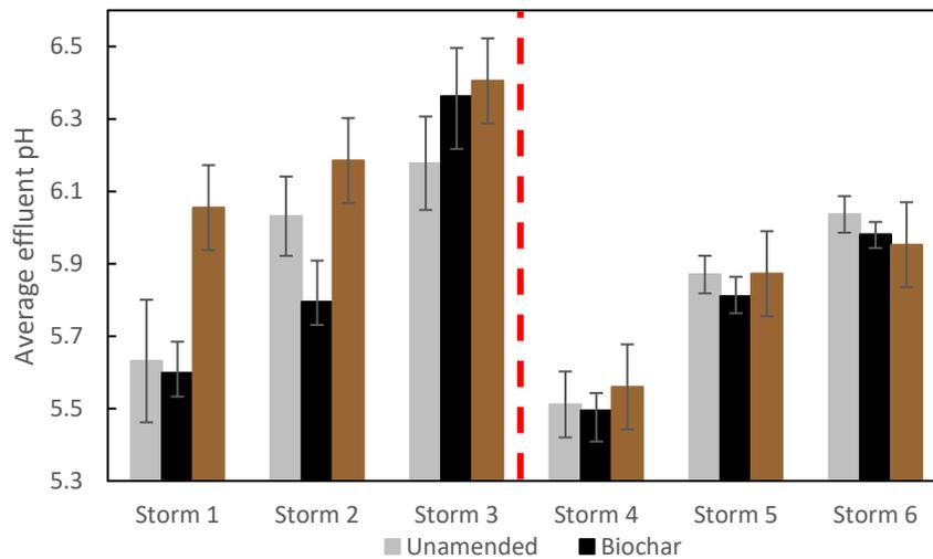
Figure 3-10: Average pH across among all soil types for six-storm series, by treatment. Columns were repacked between Storm 3 and 4. Error bars represent standard error (n=8).
