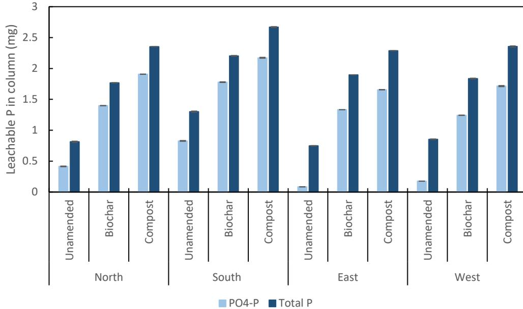
Figure 3-5: Average total mass of leachable phosphorus species in soil columns prior to storms. Error bars represent standard error (n=2).
