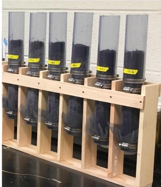
Figure 2-2 Column set-up for southern regional soil prior to stormwater application
