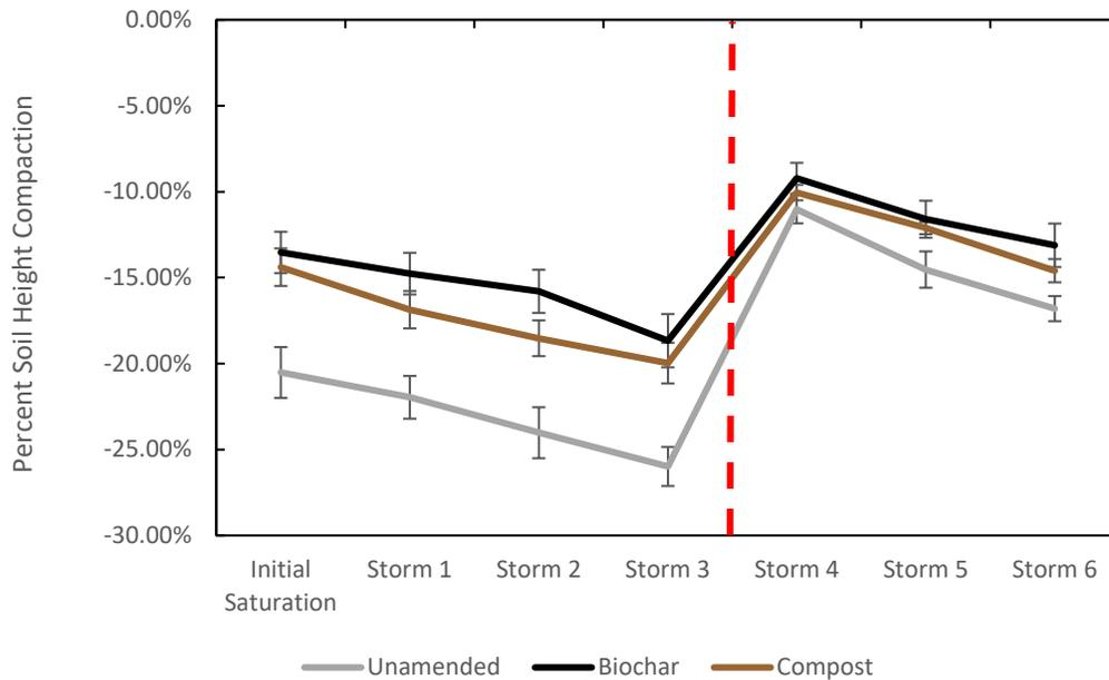
Fig 3-1: Average change in soil height from initial packed height of 30 cm, by saturation event and mixture type. Columns repacked between Storm 3 and 4. Error bars represent standard error (n=8).
