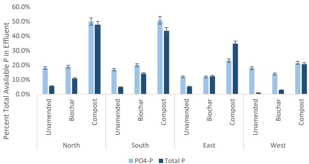
Figure 4-2: Average percent of calculated available P, including leachable and influent P, detected in effluent over six storms (cumulative)
