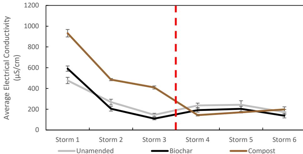
Figure 3-11: Average effluent electrical conductivity ( $\mu\text{S}/\text{cm}$ ) among all soil types for six-storm series, by treatment. Columns were repacked between Storm 3 and 4. Error bars represent standard error ( $n=8$ ).
