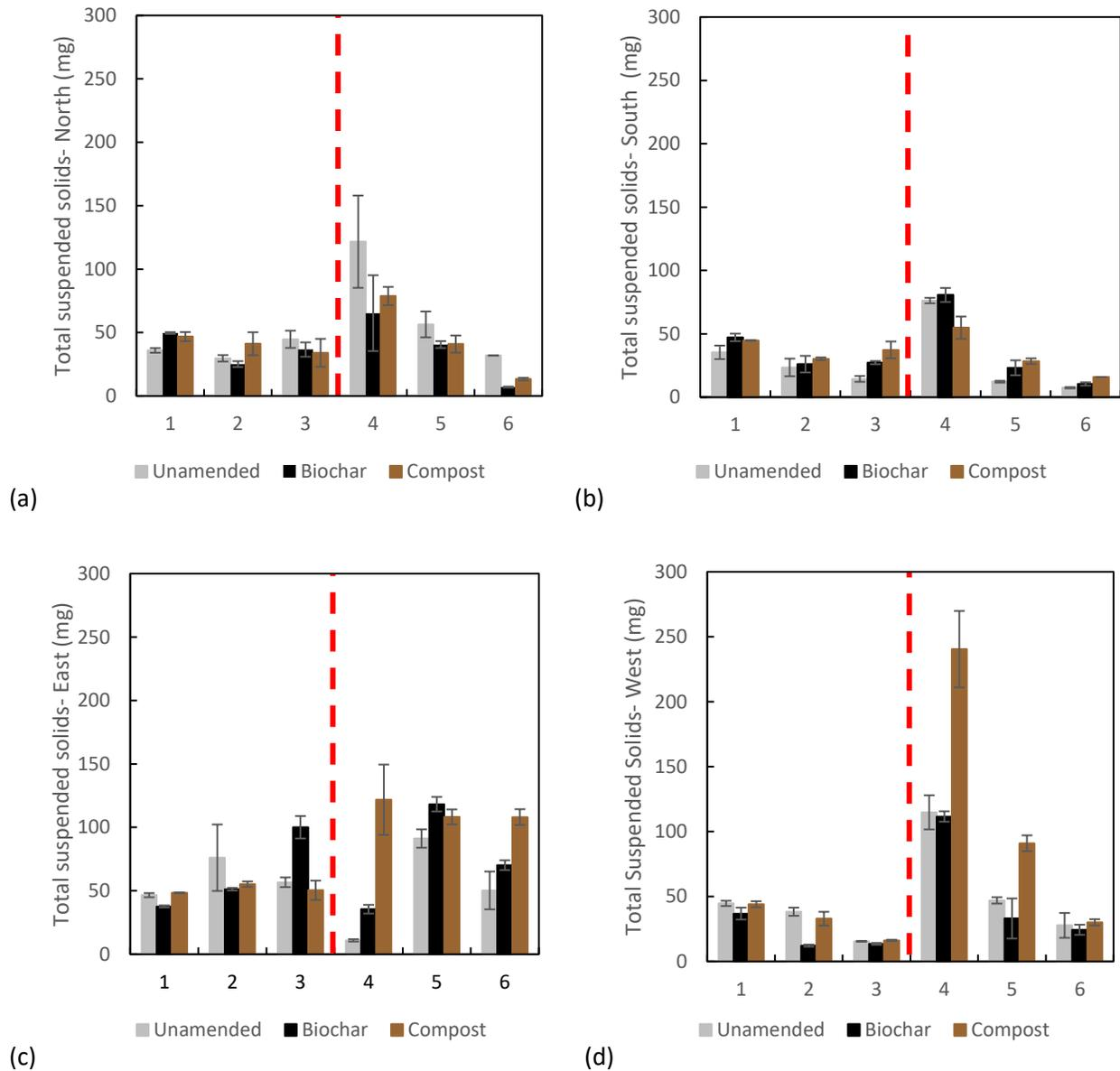
Fig 3-9: Average mass of suspended solids over 6 storm events for (a) north, (b) south, (c) east, and (d) west regional soil types. For east region (c) during Storms 2 and 3, one control column did not completely infiltrate, so filterable effluent volume was considerably less than other columns. Error bars represent standard error (n=2). Columns repacked between Storm 3 and Storm 4.
