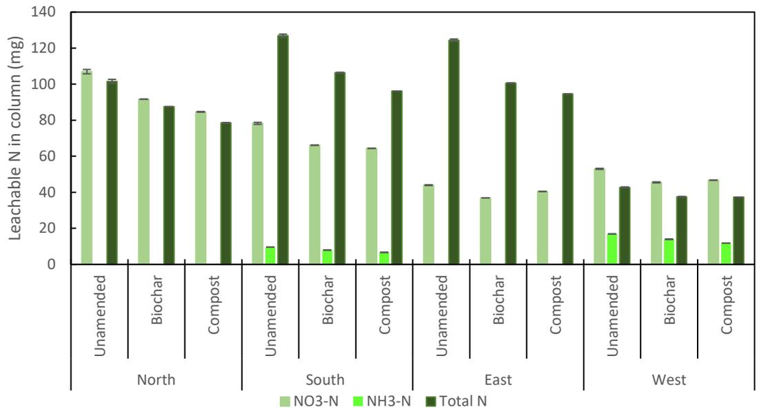
Figure 3-4: Average total mass of leachable nitrogen species in soil columns prior to storms. Error bars represent standard error (n=2).
