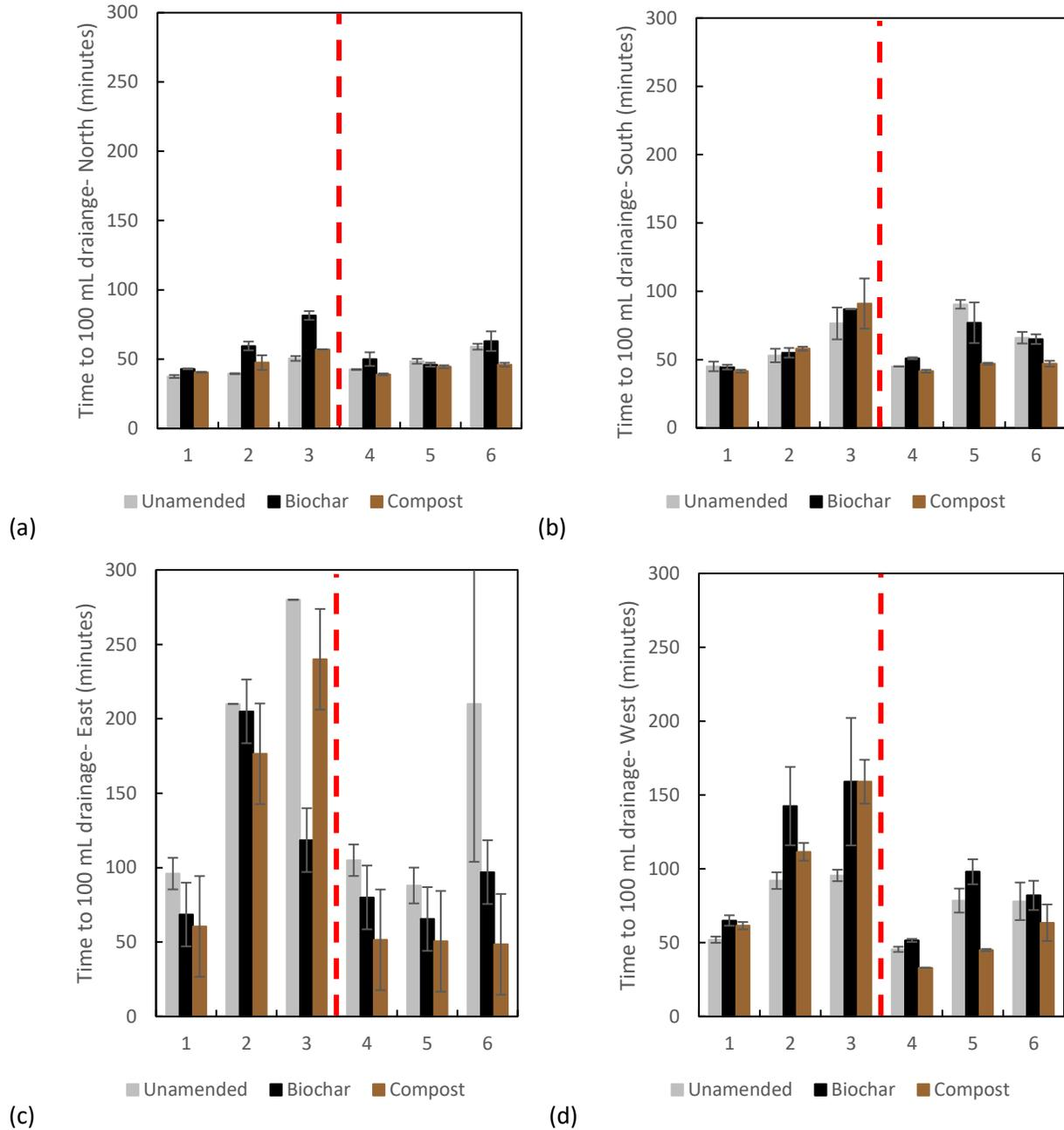
Fig 3-2: Average elapsed time from start of artificial storm to drainage of 100 mL of effluent for the (a) north, (b) south, (c) east and (d) west regional soils, by soil amendment type. Columns were re-packed between Storms 3 and 4. Error bars represent standard error (n=2 except in east region for Storms 2 and 3, in which one column did not drain 100 mL, so n=1). Columns repacked between Storm 3 and 4.
