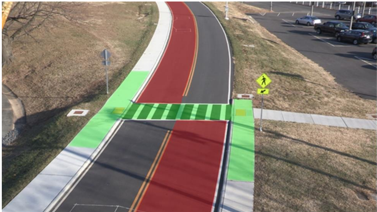
Figure 1 – The pedestrian (green) and vehicle (red) geofenced areas.
