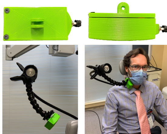
Figure 5. Prototype on a GoPro Attachment in a Hospital Setting The final vibratory device is placed on an articulating arm, which is clipped to the ENT examination chair.
