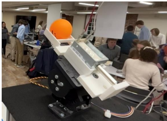
Figure 7: Solenoid Track Final Version – Mounted
