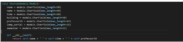
Figure 3.3.6: Course model class(Django), describing the structure of course objects used in the web app. The class includes a \_\_str\_\_ function allowing the object to be displayed as a string.
