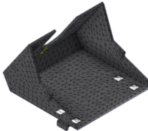
Figure 7: Custom Nexsteer EPS Mount. (Cameron Chiaramonte, 2023)
