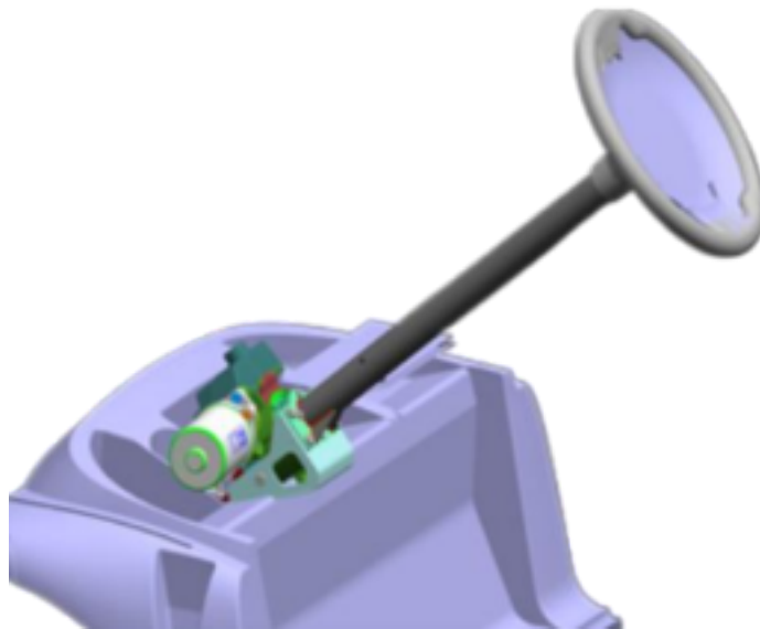
Figure 6: CAD Model of Nexteer Electric Power Steering Module. (Credit: Furukawa et al., 2018) The EPS
