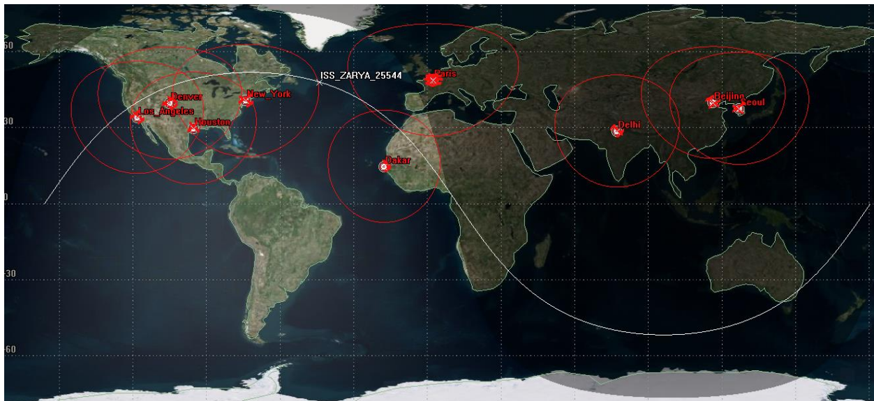
Figure 6: STK Model of Predicted CubeSat Orbit and Target Cities
