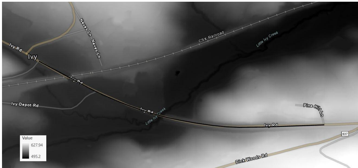
Figure 12: The DEM of the area of the bridge used to create the graph showing distance along roadway versus the elevation above sea level shown below.
