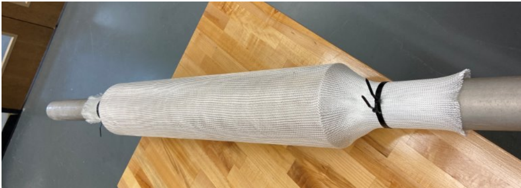
Figure 63. Fiberglass sleeve fixed over phenolic tubing.
