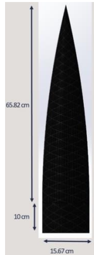
Figure 3. Final ogive nosecone design and dimensions.
