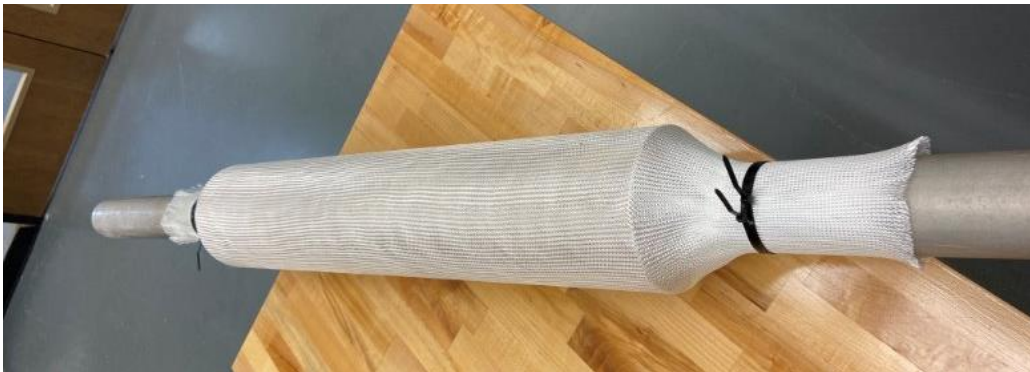
Figure 63. Fiberglass sleeve fixed over phenolic tubing.
