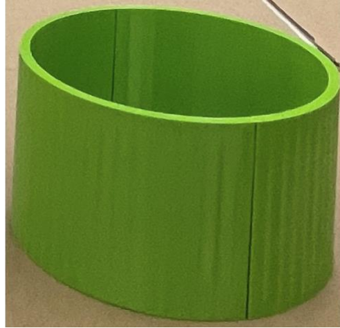
Figure 55. Extended nosecone mold (Height 10 cm)
