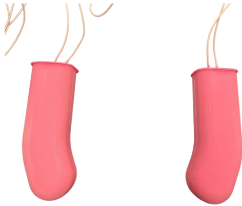
Figure 7: First Iteration Vibratory Device. This shape was designed to fit the curvature of the neck, but did not deliver the vibration to the correct location on the neck.
