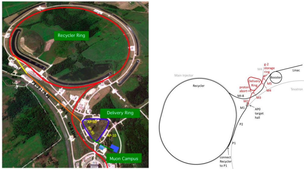
FIGURE 3.2: The diagram is the beamline to muon g-2 campus reproduced from [15]. Protons travel on black lines and muons travel on red lines.
