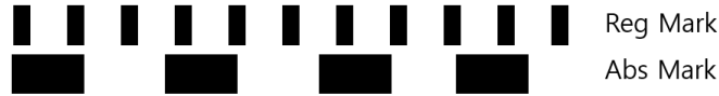
FIGURE 7.9: Two different barcode marks on the trolley track. (The drawing is Not in Scale)
