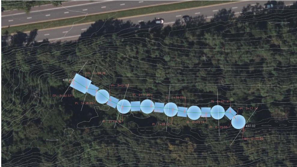
Figure 5-3. Reach 3 Design Layout
