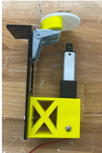
Fig. 2.6.3. First prototype of the vertical trapdoor design
