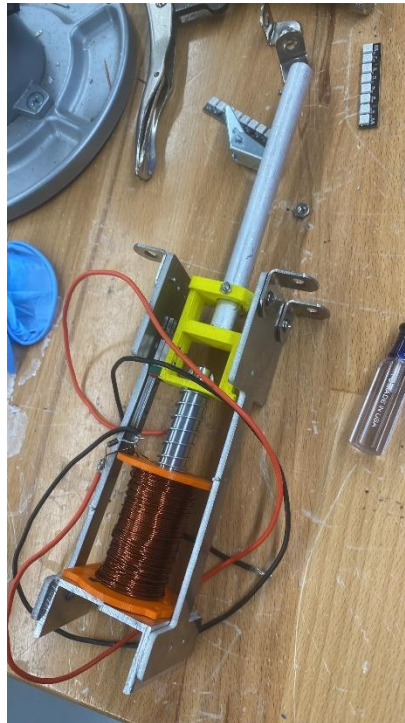
Fig. 2.3.6. Second iteration of pop bumper (pre-mounting)
