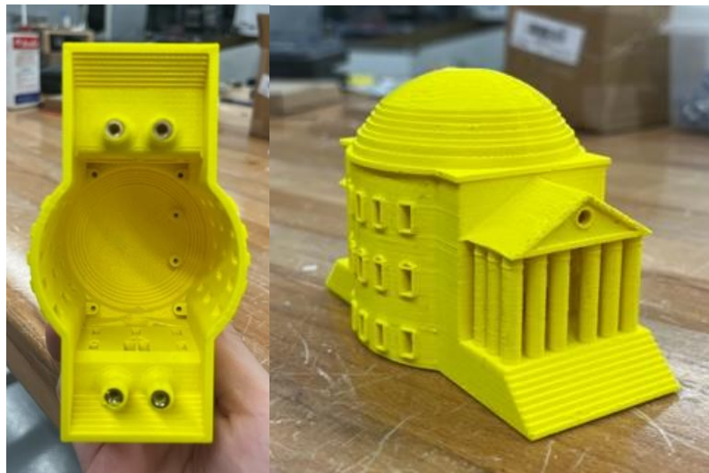
Fig. 3.1.5. Final rotunda model 3D printed to use as a place holder
