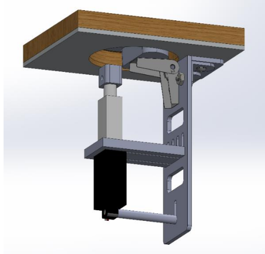
Fig. 2.6.4. Improved vertical trapdoor assembly
