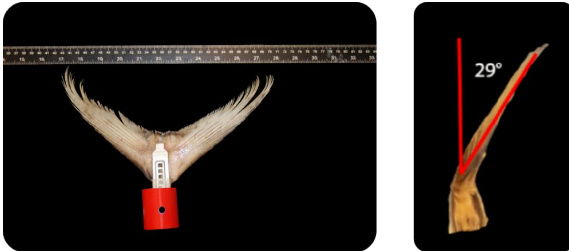
Figure 4.5 Biological sample with maximum bending angle in air about 29°. The simulation and experiment samples are modelled with similar shape and the pitch angle of caudal fin in simulation is prescribed with a smaller value due to extra resistance in water.
