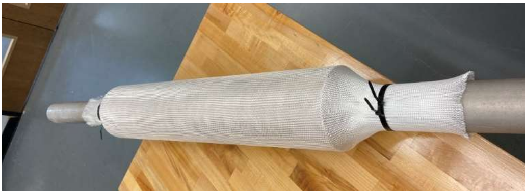
Figure 63. Fiberglass sleeve fixed over phenolic tubing.
