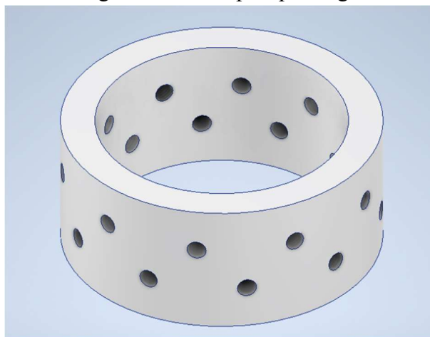
Figure 38. 2 nd Nozzle Holder Design
