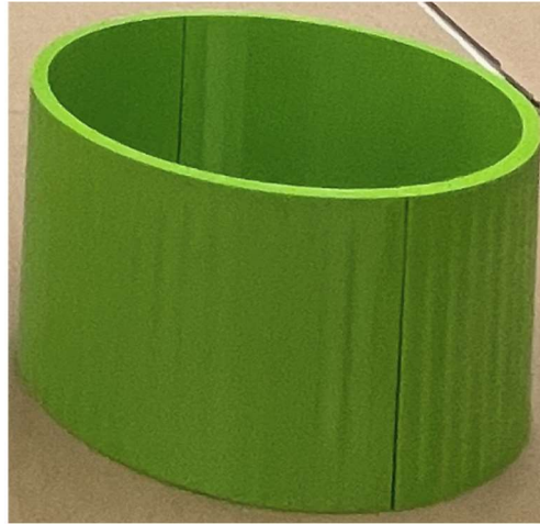
Figure 55. Extended nosecone mold (Height 10 cm)
