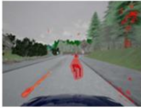
(b) Frame detected as OOD, the region in red shows the pixels responsible for deviation
