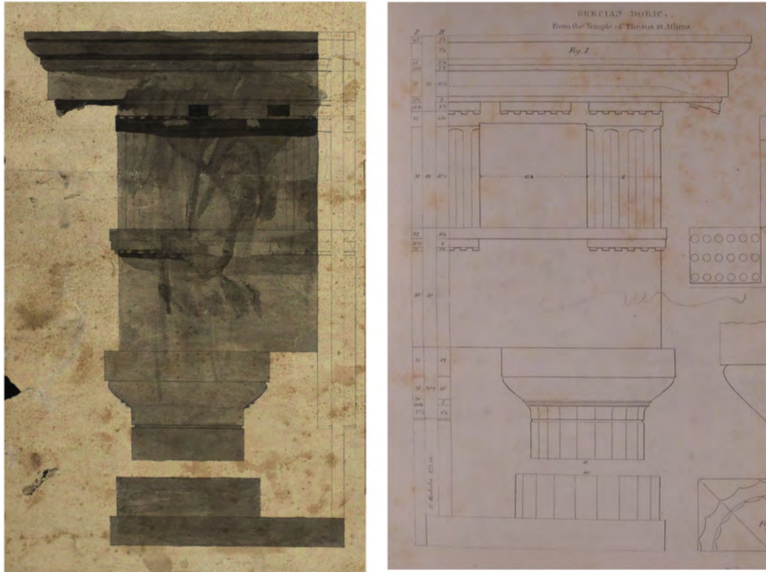
Figure 48. On the left, Weeks’s detail of MS11500 – Item 10. Weeks has drawn nearly the exact detail shown in Shaw’s pattern book. Shaw’s drawing on the right for a column and entablature of the Temple of Thesus at Athens on Plate 38, “Civil Architecture” by Edward Shaw.
