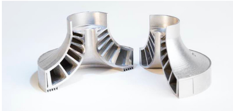
Figure 27: An additively manufactured component's complex cross section [6]
