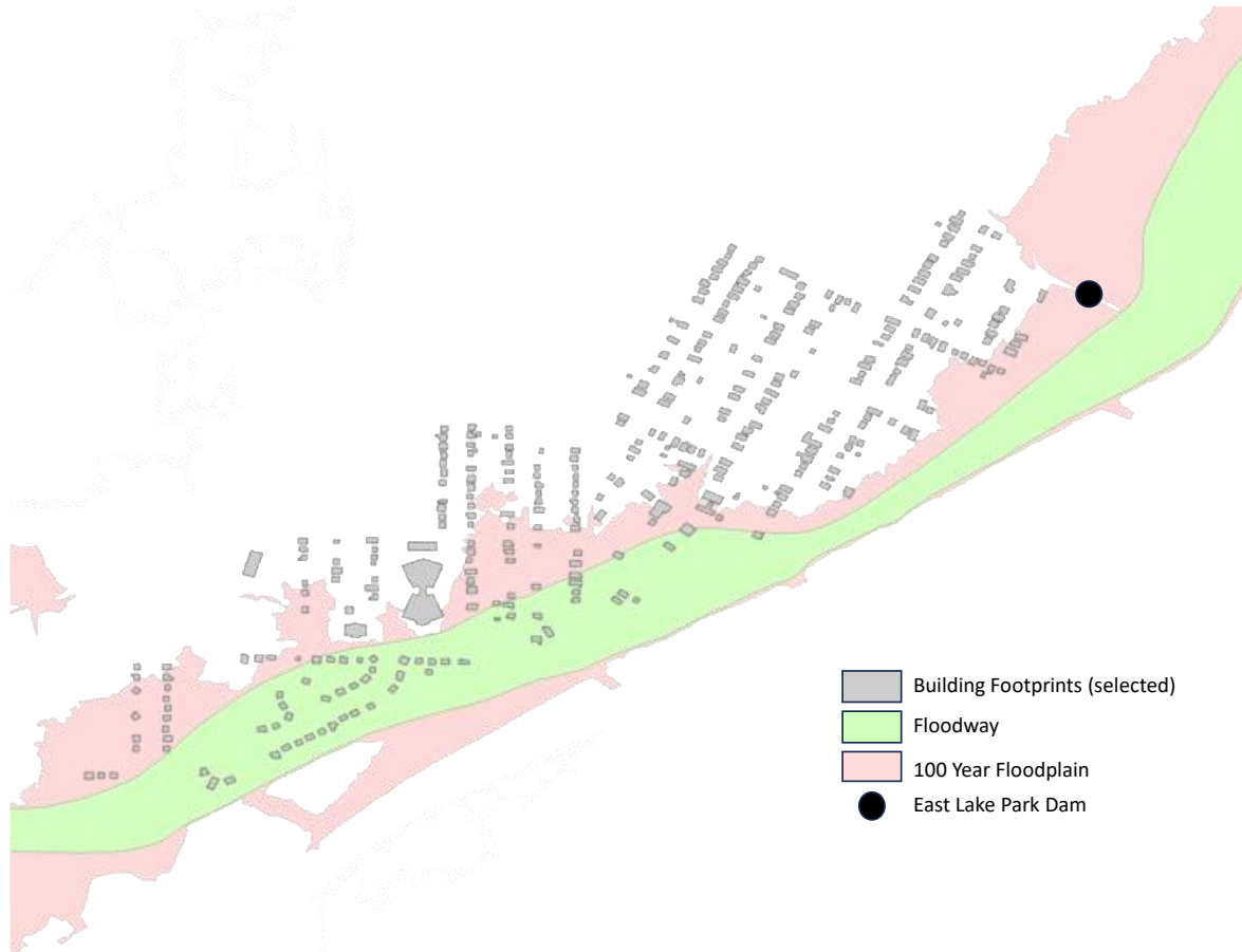
Fig. 3. Building footprints downstream of East Lake Park Dam and along floodway and 100-year floodplain [Sources: Microsoft, National Inventory of Dams, ArcGIS Online]
