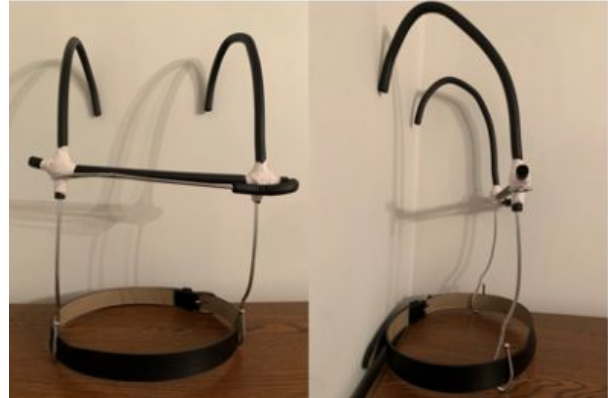
Fig. 4. Test Prototype. The test prototype was created out of a hanger and a belt to see test feasibility of the design.
