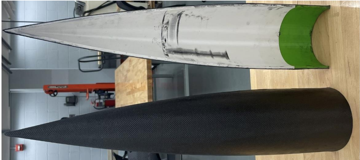
Figure 57. After 3 layers of CFRP wet layup
