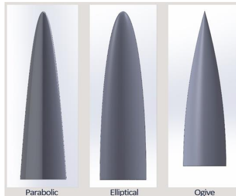
Figure 6. Image of each of the initial nosecone shapes considered
