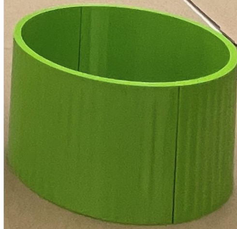
Figure 55. Extended nosecone mold (Height 10 cm)
