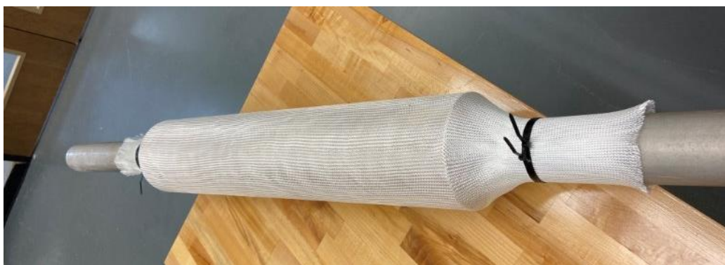
Figure 63. Fiberglass sleeve fixed over phenolic tubing.
