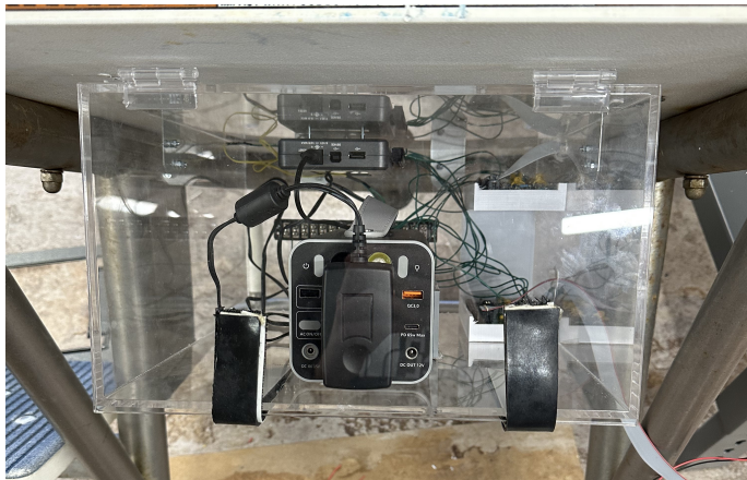
Fig. 22: Final Water-Proof Mounting Enclosure
