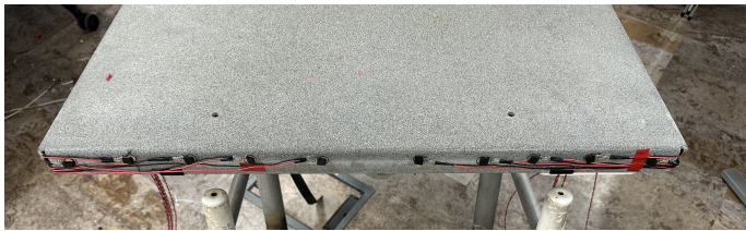
Fig. 18: Sensor Array attached to the Front Edge
