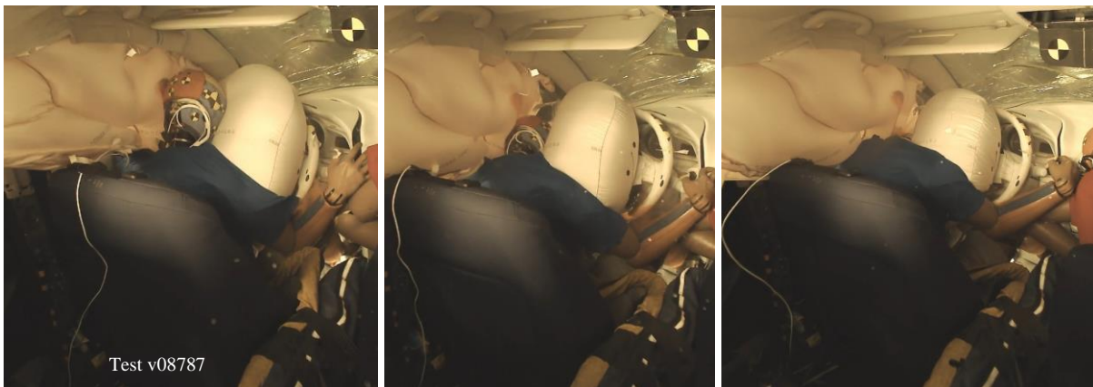
Figure 131. Video sequence (from left to right) showing head obscuration due to deployed airbags during frontal oblique crash test (images from NHTSA 2014).
