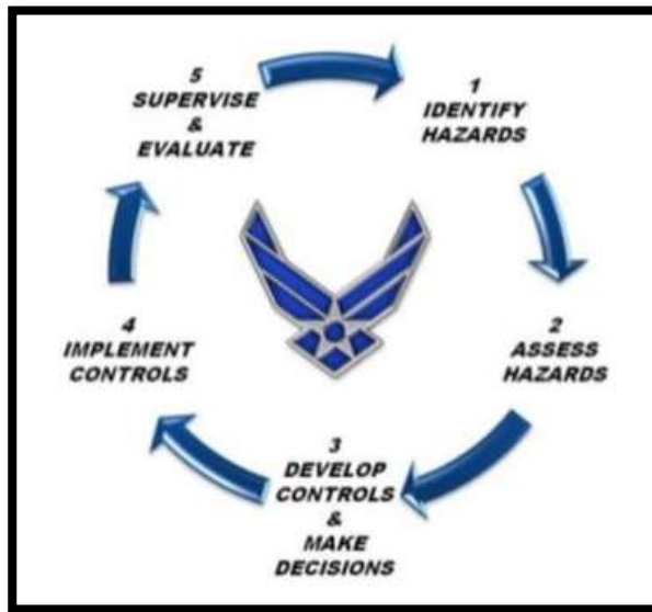
Figure 2: USAF 5-Step Risk Management Process (Rauch, 2019, p. 17) This continuous cycle of steps is used by the USAF to analyze and manage risk.
