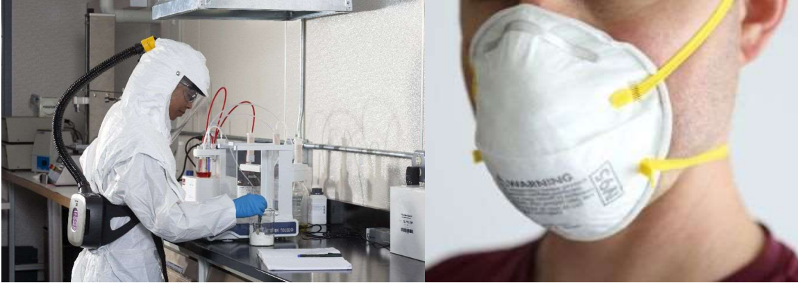
Figure 1: The left image depicts a Honeywell PAPR. The PAPR consists of the full hood, fanny pack blower, and tubing (Serban 2020). The right image shows a passive N-95 filter in use (Letzter 2020).
