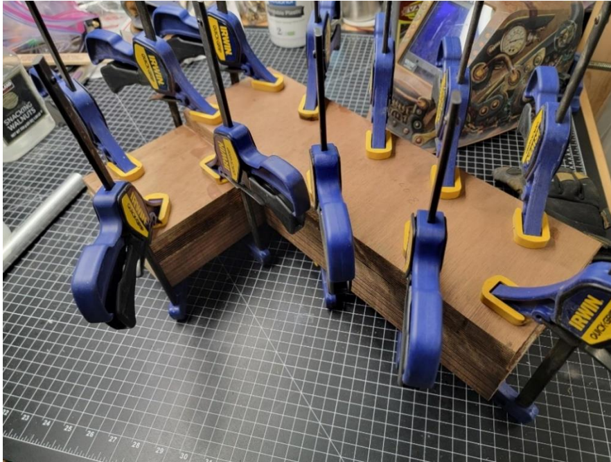
Fig. 3.3.4. Upper Playfield Plywood Stock Glued
