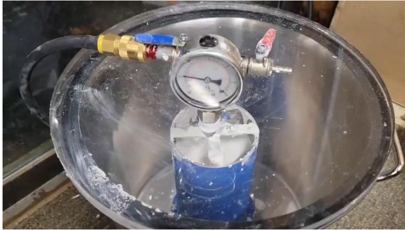
Fig. 3.1.6. Vacuum casting of wax model with plaster to create rotunda negative as a metal mold
