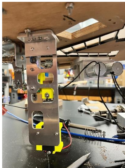
Fig. 2.7.10. Final bollard post prototype screwed into playfield
