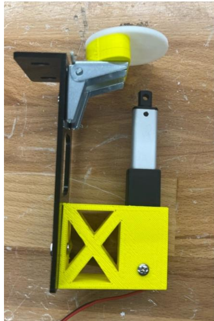
Fig. 2.6.3. First prototype of the vertical trapdoor design
