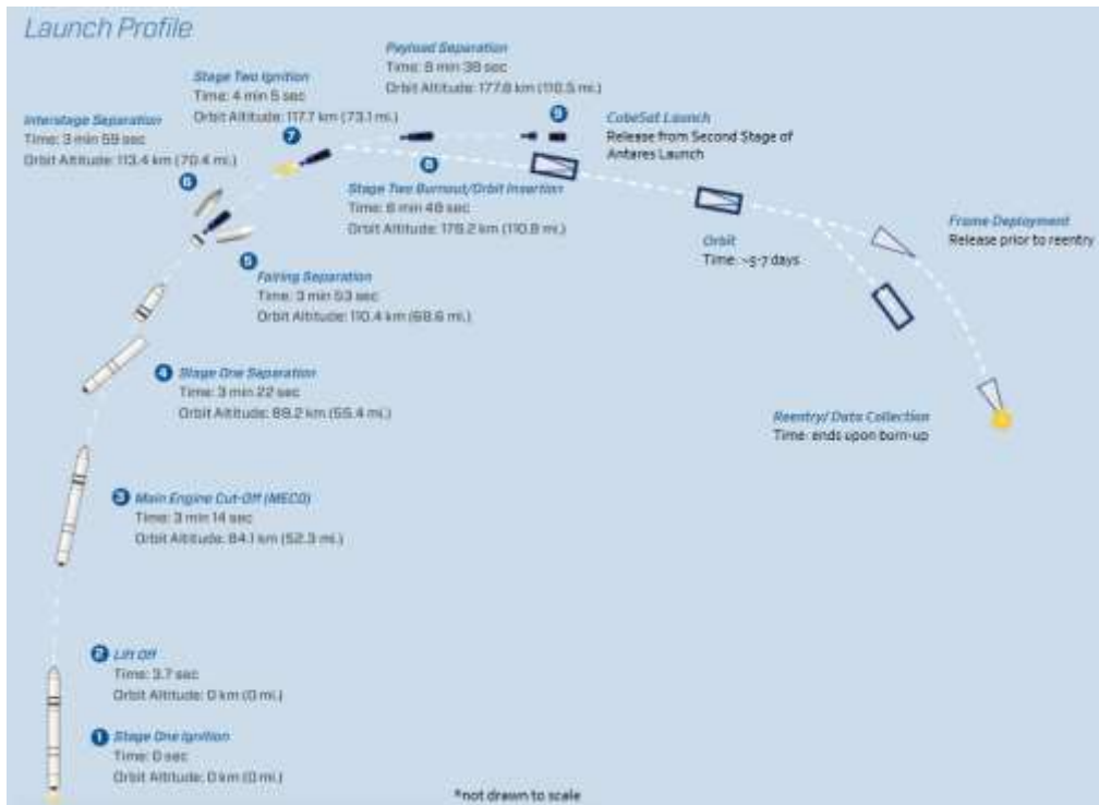
Figure 1. Diagram of Concept of Operations for CubeSat Launch to Reentry (Adapted from Clark, 2021)
