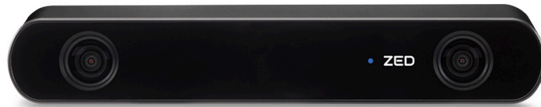
Fig. 20: ZED2 Camera Sensor
