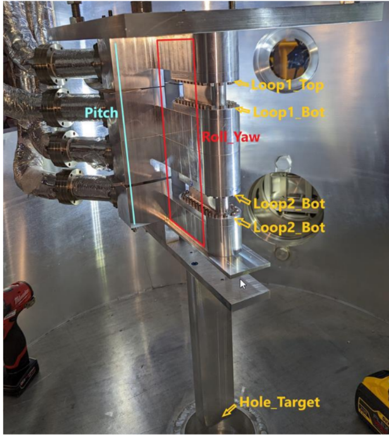
Figure 2.18: Picture of the target ladder installed in the Hall C target chamber during the alignment process from [68]. During this process, the solid target portion of the ladder only contained the hole target to prevent exposure of the other targets to air.
