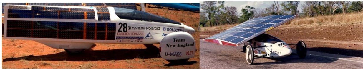
a) Good aerodynamics but poor solar array design
